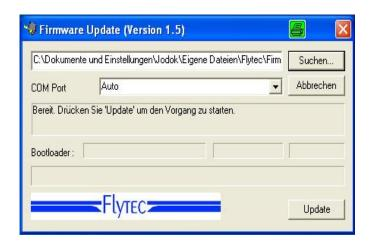
Now connect the USB cable with the instrument. Afterwards you can set the interface in the field Com Port, or if it is unknown to you, set to **Auto** and have thereby an automatic search prompted. The virtual COM interface should be positioned between 1 and 8. Above this value the Flasher can no longer recognise the interface.
